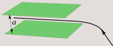
Beam trajectory passing through a bending magnet. In the straight part of the orbit after the exit there are two parallel metal plates (shown by green color).
