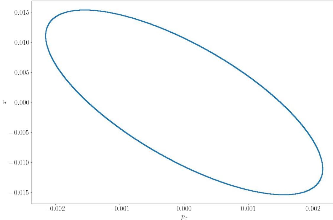
To show stability, track through a field map with perfect linear forces for 1M turns through the FODO lattice.
