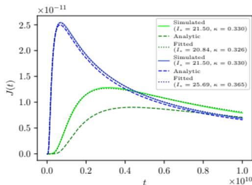
Outgoing current of a Fokker-Planck process (continuous lines), compared with the analytical approximation (dashed lines); dotted lines are a fitting procedure of  $\kappa$  and  $I_*$  based on the analytical approximation.
