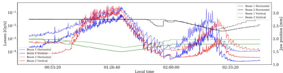
[From Gorzawski et al.] Beam losses in LHC from the IC-BLM monitor. The losses are measured via moving jaws that perform the scraping on the vertical and horizontal plane separately. These measurements have been used to probe the local diffusive regime of beam halos.
