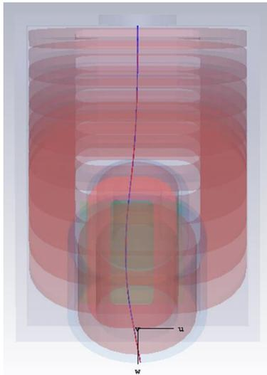
vertical magnetic field on ion path
