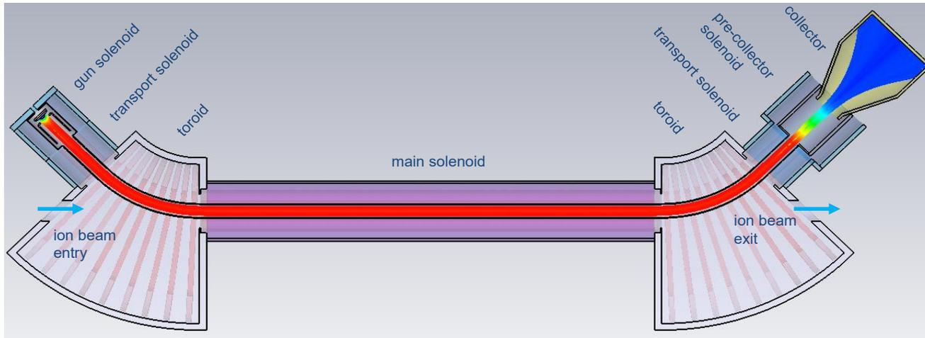
Magnetic field along the SCC electron lens
