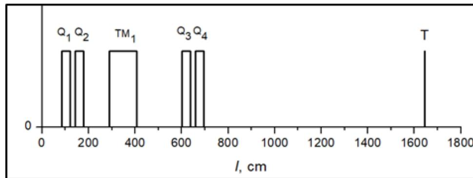
Figure 2: New scheme of the beam line #1. Here Q1-4 are quadrupoles, TM1 is the bending magnet, T is a target
