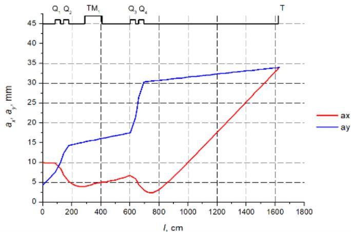
Figure 3 : Horizontal (red curve) and vertical (blue curve) envelopes of the ion beam  $^{209}\text{Bi}^{38+}$
