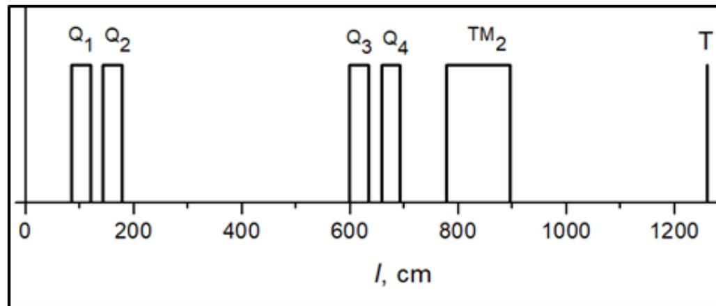
Figure 5: Scheme of the beam line #2. Here Q1-4 are quadrupoles, TM2 is the bending magnet, T is a target
