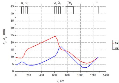
Figure 6 : Horizontal (red curve) and vertical (blue curve) envelopes of the ion beam  $^{197}\text{Au}^{26+}$
