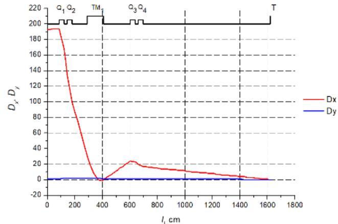
Figure 4: Horizontal dispersion function  $D_x$  (red curve) and vertical dispersion function  $D_y$  (blue curve) of the ion beam  $^{209}\text{Bi}^{38+}$
