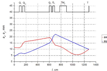
Figure 8 : Horizontal (red curve) and vertical (blue curve) envelopes of the ion beam  $^{132}\text{Xe}^{16+}$
