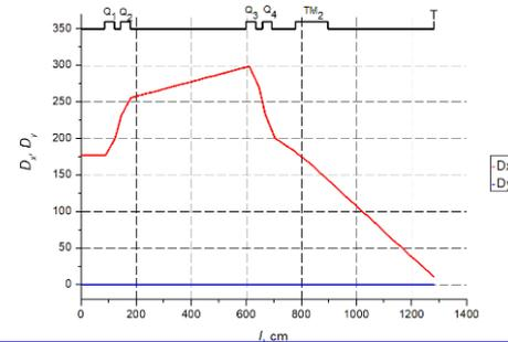
Figure 9: Horizontal dispersion function  $D_x$  (red curve) and vertical dispersion function  $D_y$  (blue curve) of the ion beam  $^{132}\text{Xe}^{16+}$
