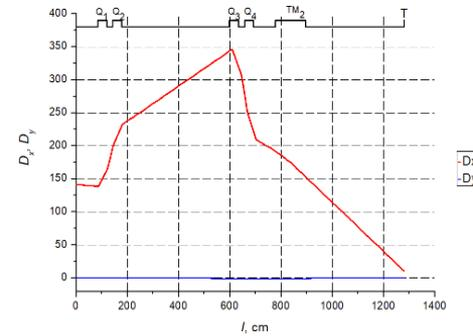
Figure 7: Horizontal dispersion function  $D_x$  (red curve) and vertical dispersion function  $D_y$  (blue curve) of the ion beam  $^{197}\text{Au}^{26+}$
