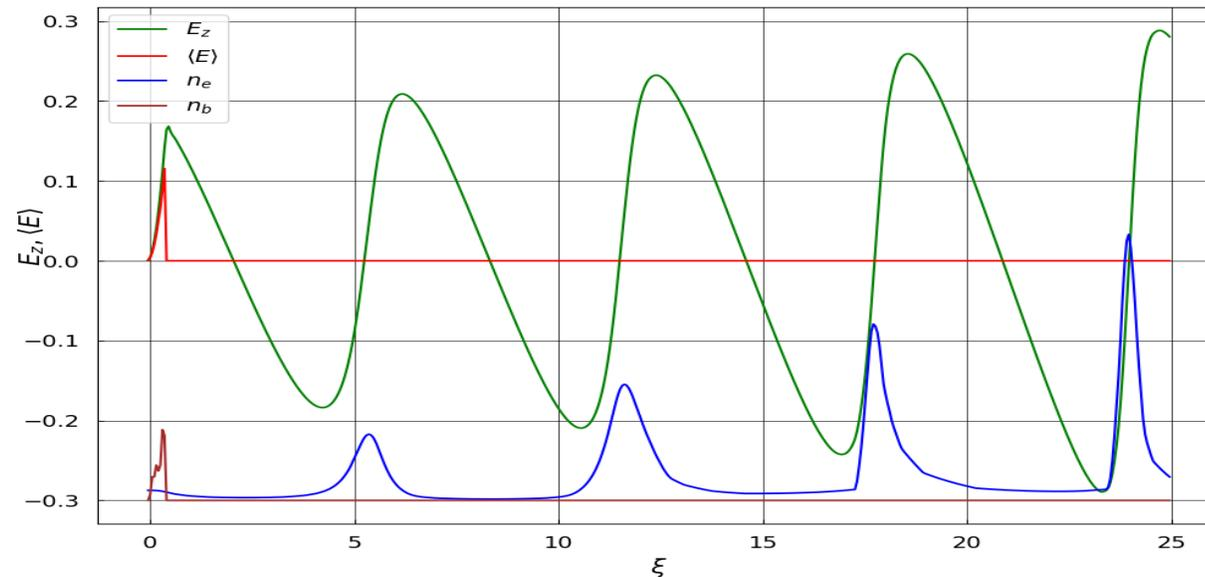
An example of the excitation of such a field by a short electron bunch, with a charge distributed along the cosine, from minimum to maximum values.
