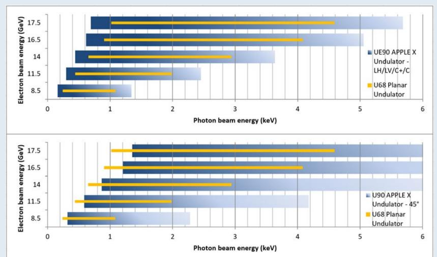
Figure 3: Photon energy ranges generated by helical UE-90 and planar U68 undulators. The upper figure shows the case of vertically and horizontally as well as circularly polarized modes. The lower figure illustrates the case with linear polarization at an angle of 45°
