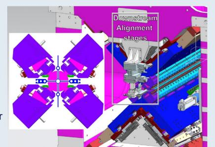
Figure 4: Layout of the alignment stages and a cross-section of the vacuum chamber surrounded by four magnetic structures at the minimum gap.
