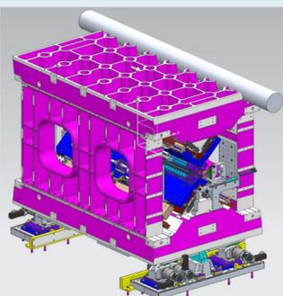
Figure 2: UE90 frame with a cutout for the SLRS system
