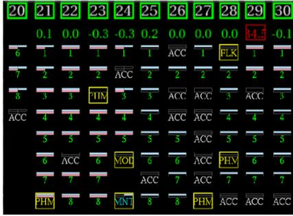
Klystron CUD (Overview) Panel showing the status of all the LCLS klystron. Whether they are on for the beam going to the hard x-ray line (blue) and/or soft x-ray line (red) is indicated by horizontal, coloured bars, in this case 10.7 and 4.7 GeV in Dual Energy Mode. The yellow boxes indicate problems, like PHM (Phase Mean), Modulator, Maintenance, or stations with ACC ready to be used for acceleration.
