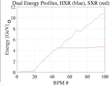
Energy Profile along the Linac. For hard x-rays (HXR) it is 10.7 GeV, while for soft x-rays (SXR) it is 4.7 GeV at the end.
