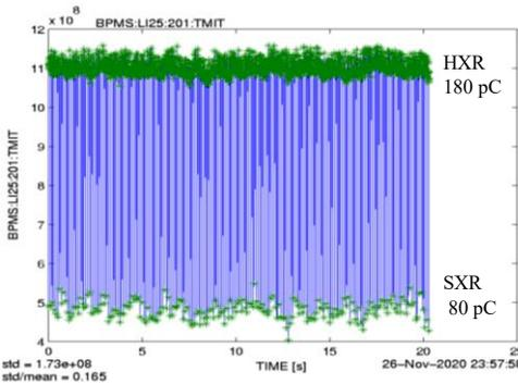
Cutting charge in Bunch Compressor 1 (BC1) for HXR the typical 250 to 180 pC, while for SXR it is down to 80 pC (or even 30 pC), see below.
