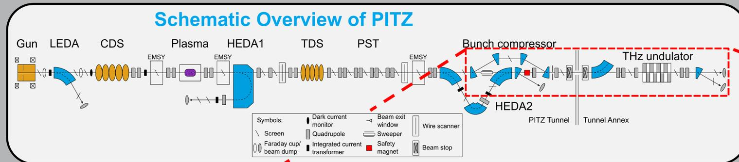
In order to allow THz pump--X-ray probe experiments at full bunch repetition rate for users at the European XFEL, the Photo Injector Test Facility at DESY in Zeuthen (PITZ) is building a prototype of an accelerator-based THz source. The goal is to generate THz SASE FEL radiation with a mJ energy level per bunch using an LCLS-I undulator driven by the electron beam from PITZ. Therefore, the existing PITZ beam line is extended into a tunnel annex downstream of the existing accelerator tunnel.
