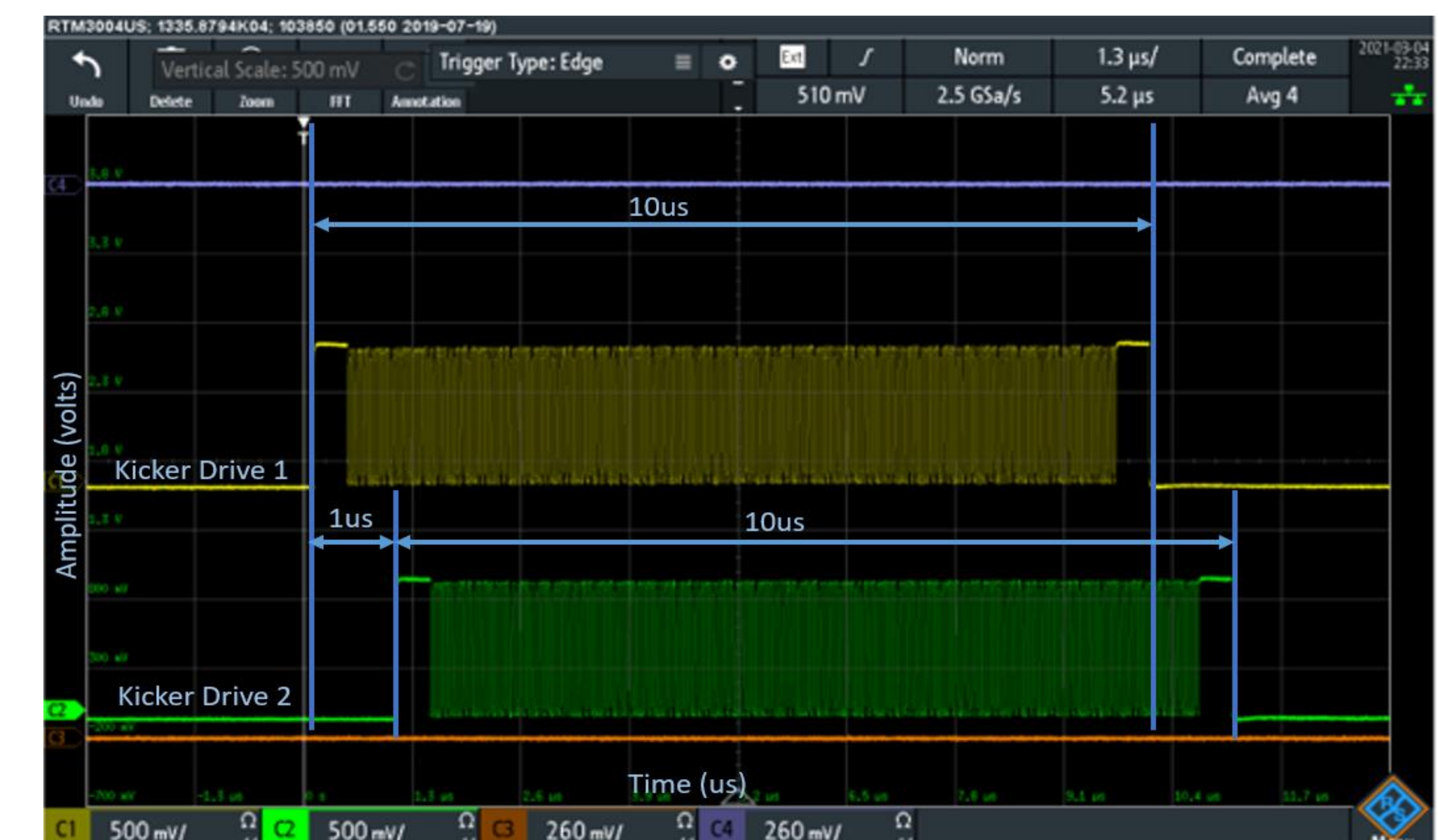
BPG output channels, CH2 delayed by 1us compared to CH1
