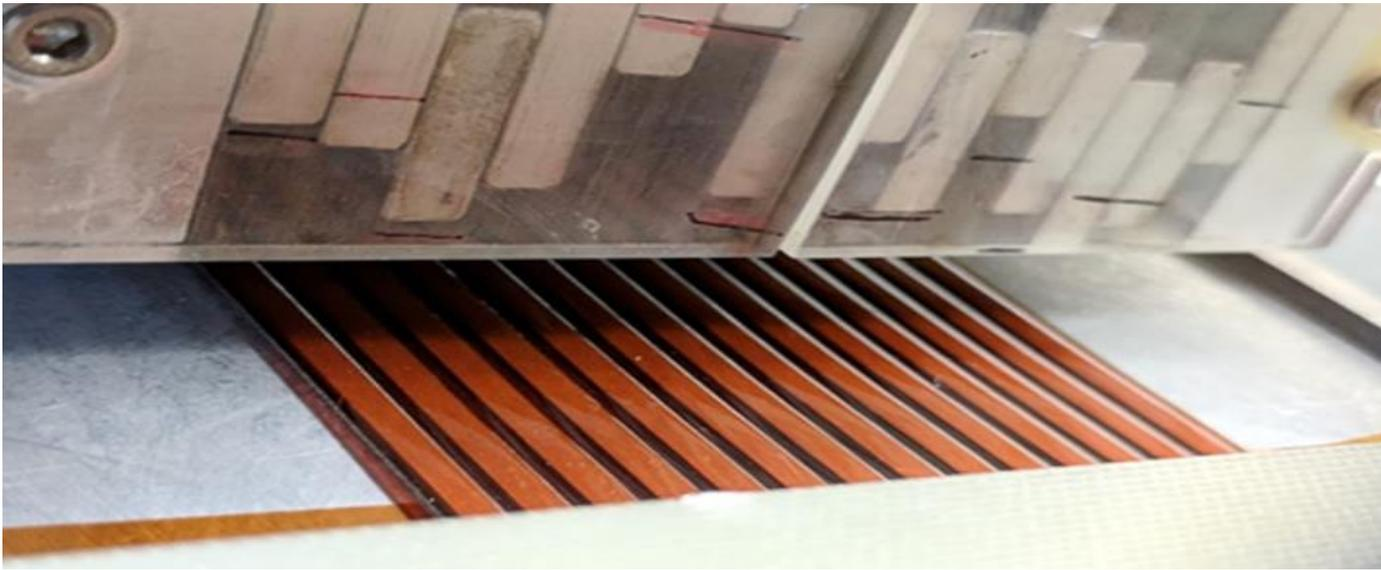
Twenty-eight flat wires installed in the EPU 56 of the storage ring of the accelerator Taiwan Light Source (TLS)
