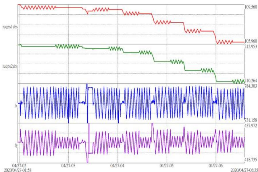
The quadrupole magnet is composed of electromagnets, so we must first understand how the current setting of the quadrupole magnet responds to a variation of the working tune.
