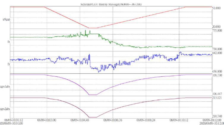
The hysteresis characteristic of the quadrupole magnet causes an error of the magnetic-field distribution. When the current setting alters significantly, the working tune of the storage ring has an offset error 25 kHz
