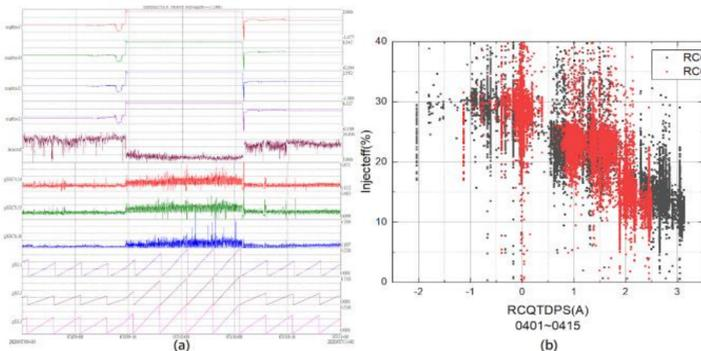
For a current working tune feedback system, we can adjust the current value of the trim coil on the local quadrupole magnet to correct the offset error. We use an asymmetric magnet current setting to correct the working tune. If the current setting is greater than 1.5 A, there is a risk, however, of increasing the radiation dose and decreasing the injection efficiency.
