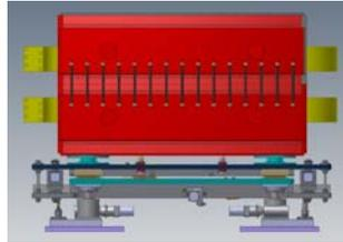
Fig. 1 Structure of dipolar girder system with the vibration isolator
