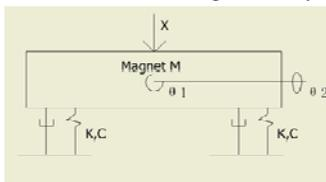
Fig. 4 Dynamic model of magnet support system
