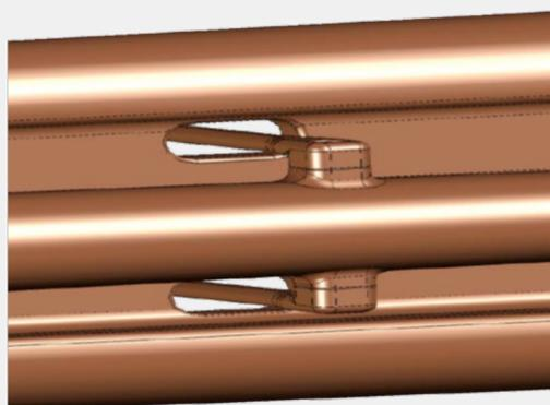
Pair of electrodes with stabilizers and opening in the other electrode pair for the bridging
