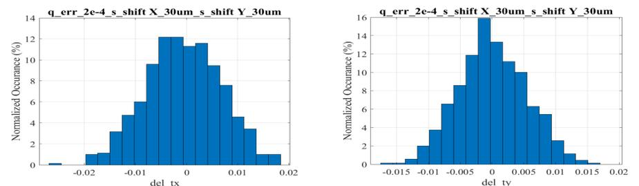
Figure 4: The tune-shifts with the 30 μm misalignment of sextupoles and the 0.02% field errors of quadrupoles (700 seeds).
