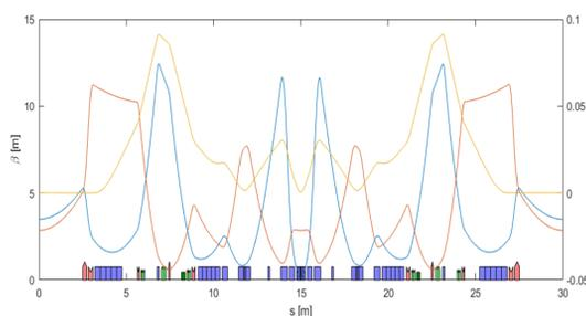
Figure 1: Layout and optical functions of the candidate lattice designed for the SAPS. The blue, red, green, dark green blocks represent dipoles, quadrupoles, sextupoles and octupoles, respectively.
