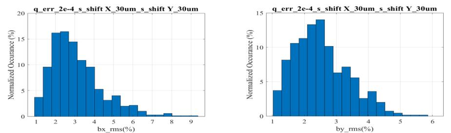
Figure 3: The RMS distribution of the beta-beatings with the 30 μm misalignment of sextupoles and the 0.02% field errors of quadrupoles (700 seeds).
