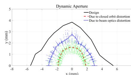
Figure 5: DA tracking result. (Black line): bare lattice DA; (red dot): 50 cases tracking result with closed orbit distortion; (red line): average DA with closed orbit distortion; (blue dot): 50 cases tracking result with beam optics distortion; (blue line): average DA with beam optics distortion.
