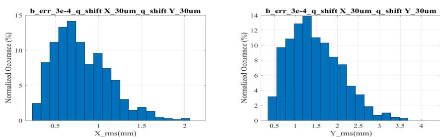
Figure 2: The RMS distribution of the closed orbits with the 30 μm misalignment of quadrupoles and the 0.03% field errors of dipoles (700 seeds).
