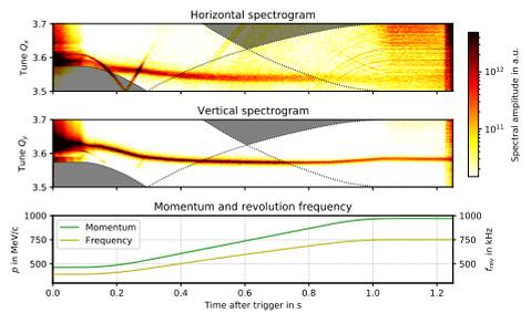
Figure 3: Evolution of the tune as bold line in the frequency spectrograms during bunching and acceleration of a deuteron beam to 970 MeV/c. The dashed lines indicate the excitation frequency band; regions outside the band are shaded.
