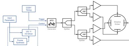
Figure 1: Signal-flow graph of the noise excitation system
