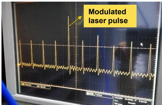
The photodetector signal converted from laser pulse of EOM
