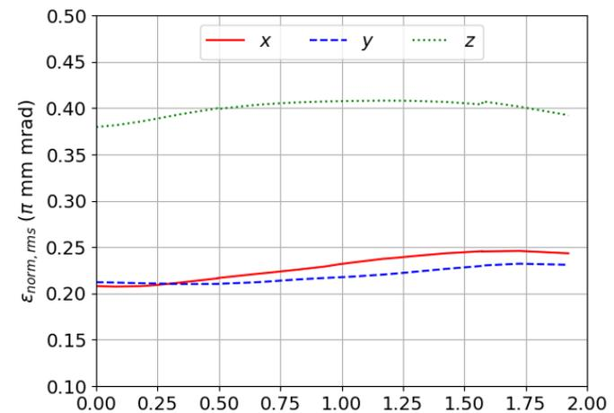
Figure 5 :Normalized rms emittance along the MEBT.
