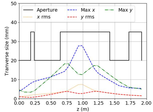
Figure 4 :Maximum and rms beam size on the transverse plane in the MEBT. The aperture is the physical radius of the elements that composed the MEBT.
