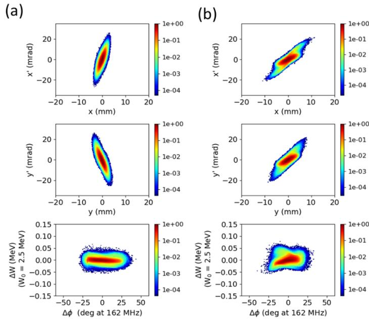
Figure 3: Phase space distribution at the entrance (a) and at the end (b) of the MEBT.
