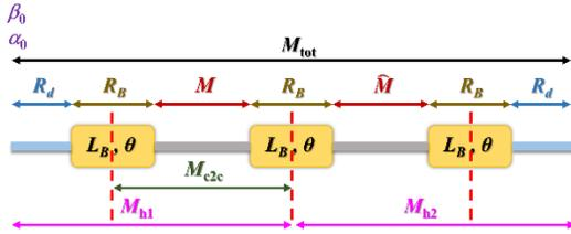
Fig. 1 Schematic of the TBA structure with three identical dipole magnets of length  $L_B$  and bending angle  $\theta$ .
