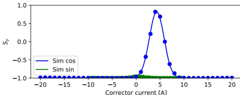
To correct the orbit harmonic  $h=4$ ,  $[\sin 4, \cos 4] = [2.797, 0.669]$  and to spin-flip:  $h=5$  currents are  $[\sin 5, \cos 5] = [10.0, -18.0]$  and  $I_{max} = 23.086$ .
