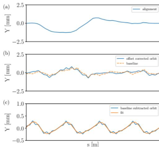
This example orbit at  $|G\gamma| = 8$  has a corrector current with respect to h=8 of  $\cos 8\nu=5$  A,  $\sin 8\nu=13$  A. The components of the fit results are:  $[\sin 4, \cos 4, \sin 5, \cos 5, \sin 8, \cos 8]=[0.1997$  mm, 0.07796 mm, 0.01137 mm, 0.00031849 mm, -0.01263 mm, -0.04177 mm].
