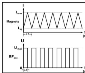
Triangular cycling with fast extraction (AC+DC 14.5 kW)
