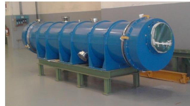
Fast ramped SIS300 Dipole in Cryostat
