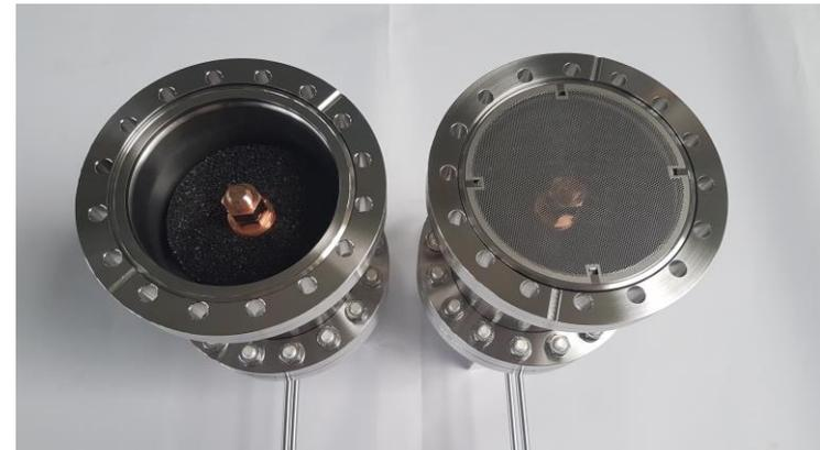
Cryogenic adsorption pumps
