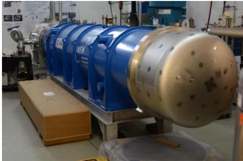
Set-up of full size SIS300 dipole magnet at test stand t ILK
