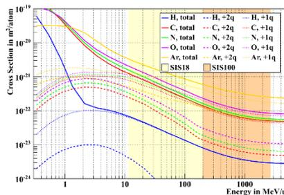
Cross section for charge exchange
