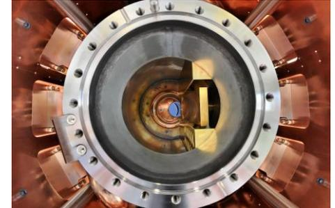
Cryogenic ion catchers with low desorption surface
