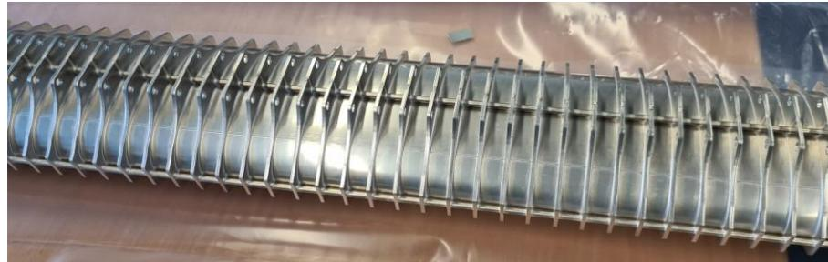
Actively LHe cooled, thin wall magnet chambers
