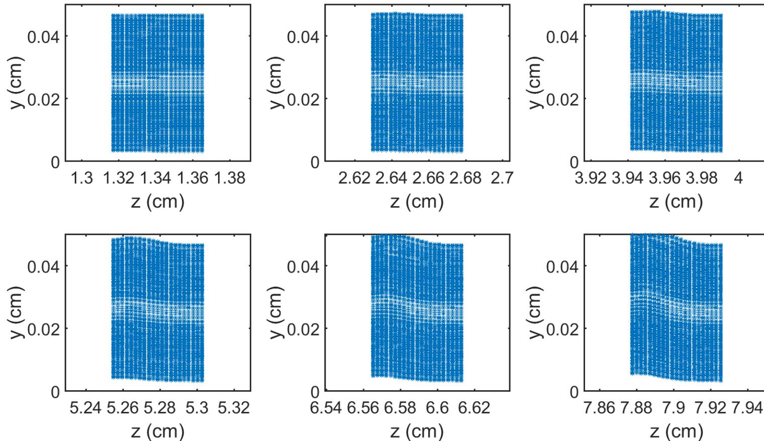
**Dynamics of the off-axis bunch on the  $y - z$  plane. Vertical axis limits correspond to half of **vacuum channel** width, horizontal axis limits correspond to the frame around the bunch. The initial vertical offset of the bunch is 0.25 mm, the length of the structure is 8 cm.**
