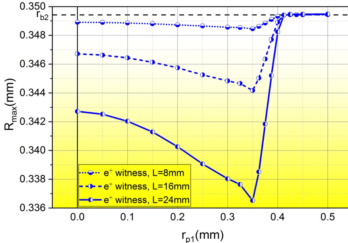
Changing  $r_{p1}$  from 0 to 0.35mm (positron bunch radius) leads to an improving of test bunch focusing. At  $r = r_{p1}$  is maximal focusing. When size of vacuum channel is greater than transverse bunch size there is disimproved.
