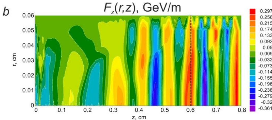
$t=26.69ps$ : drive electron bunch is at the output end of the waveguide (8mm)
