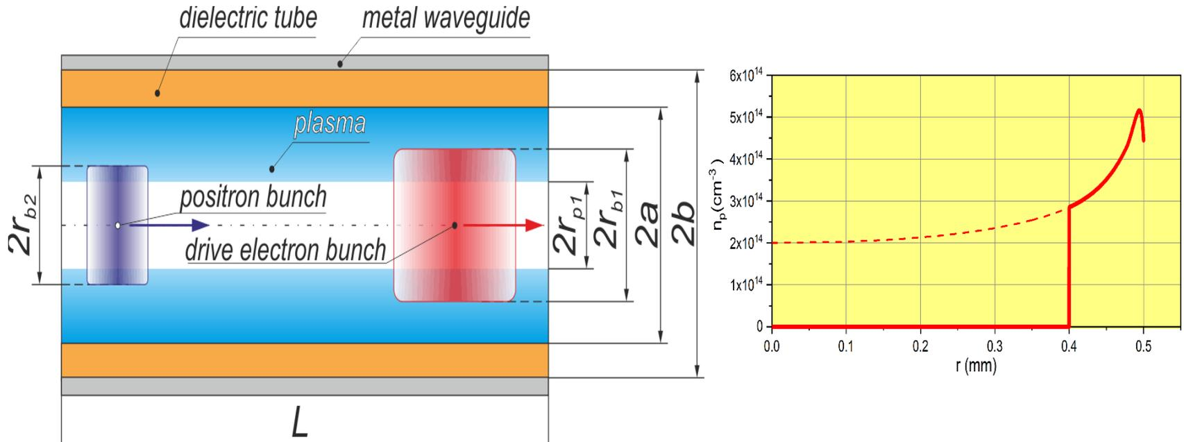
The sketch of the PDWA. Orange area shows dielectric tube, Drift channel of size  $2a$  is partially (inner radius  $r_{p1}$ ) filled with radially inhomogeneous plasma [blue color, the profile is at the right, Bobrova N.A. et al. PRE, 65, 016407 (2001)]. Drive bunch is pink cylinder and positron bunch is purple cylinder
