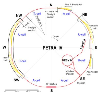
Layout of PETRA IV. The positions of undulator cells (U-cell) and relaxed cells (A-cell) for the combi lattice arcs are marked in blue. The pure HMBA lattice is using U-cells for all arcs.
