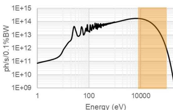
Figure 3: Photon flux density at 5.2 mm gap.
