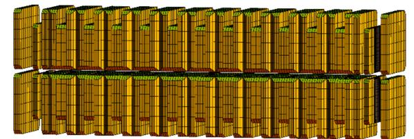
Figure 1. AVS-US Magnetic model generated by RADIA. Yellow parts are NdFeB magnets. Overall length is 0.3625 m, total width is 72 mm, overall height is 125.2 mm (including gap) and minimum gap is 5.2 mm.
