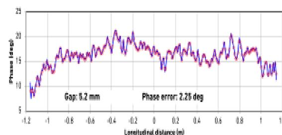
Phase error is  $<2.5^\circ$  at minimum gap
