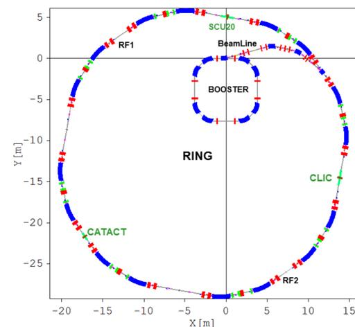
Model of the KARA ring, Booster and Beam Line [2]. Magnets are depicted in blue, quadrupoles in red and sextupoles are marked in green.
