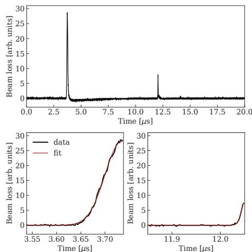
Figure 1: Top: Example of BLM15 signal  $\ell_m(t)$  recorded in SS15. The losses generated by the island sweeping through the blade of the dummy septum cause the first spike, the second one represents the losses of the core. Bottom: detailed views of the island and core losses (left and right plot, respectively) together with a fitted Gaussian model (from [5]).
