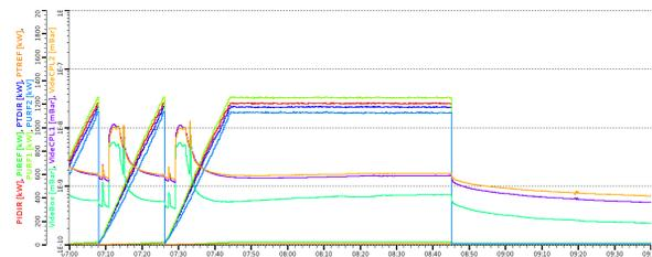
Figure 2: Typical RF conditioning of couplers with vacuum and power measurements.
