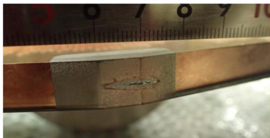
Figure 2: Photo of the collimator jaw severely damaged by the beam entering from the left and exiting to the right.
