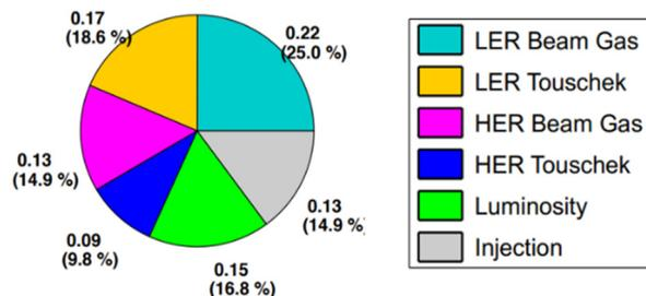
Figure 3: TOP background rates (and fractions) measured by machine studies in 2020 June, with beam currents of  $\sim 500 \text{ mA}$ , 978 bunches, and  $\beta_y^* = 0.8 \text{ mm}$ .
