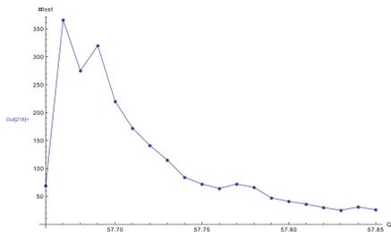
Figure 5: Particle losses through the 18 GeV RCS acceleration cycle as a function of horizontal tune. The initial bunch parameters were RMS  $dp/p = 4.3e-3$ , and bunch length of 71 ps RMS.
