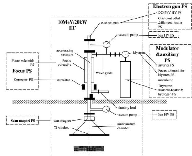
Figure 1: Power supply system of the IIF.
