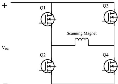
Figure 3: H-bridge converter for scanning magnet.
