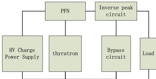
Figure 9: Linear modulator.
