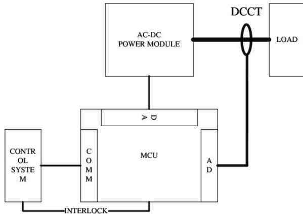
Figure 2: Unipolar DC power supply.
