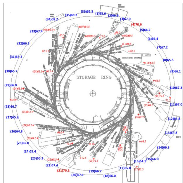
Figure 1: Hand held noise meter mapping.
