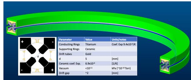
Figure 1: Circular Radio Frequency Quadrupole. Four flat vanes are precision shaped and fitted into ceramic guides. Drift tubes are distributed around the ring and are used for orbit correction and can be used to accelerate the beams. This design is modeled on the PALLAS CRFQ [10].
