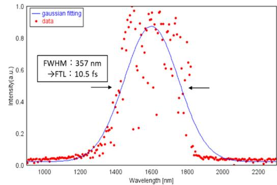
Figure 4: Spectrum after the amplifier.
