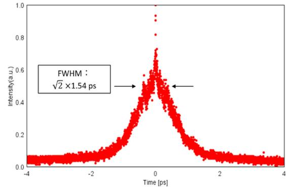
Figure 3: Autocorrelation trace after the amplifier.
