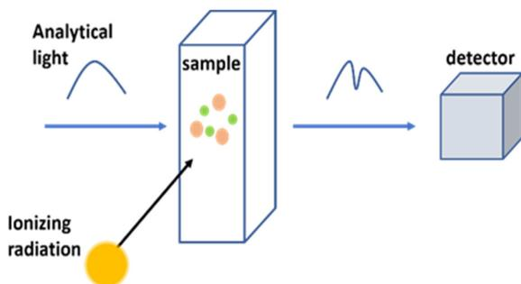
Figure 1: Schematic of pulse radiolysis.
