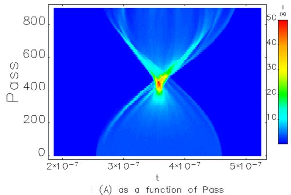
Figure 3: Simulated beam instabilities with ELEGANT.
