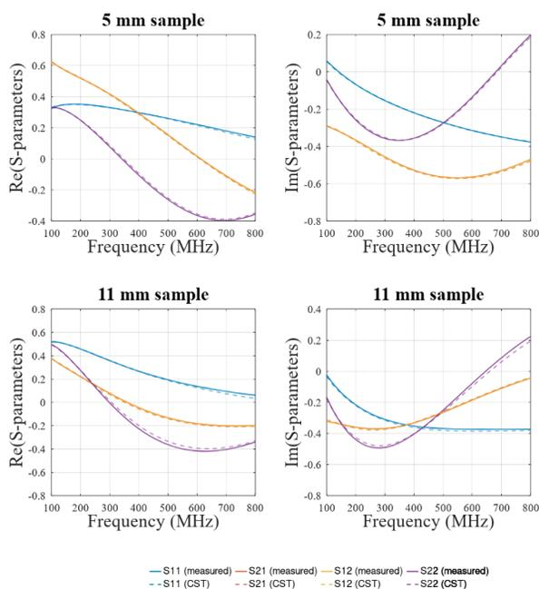
Figure 4: S-Parameters, measured field (solid lines) compared with CST simulated model.
