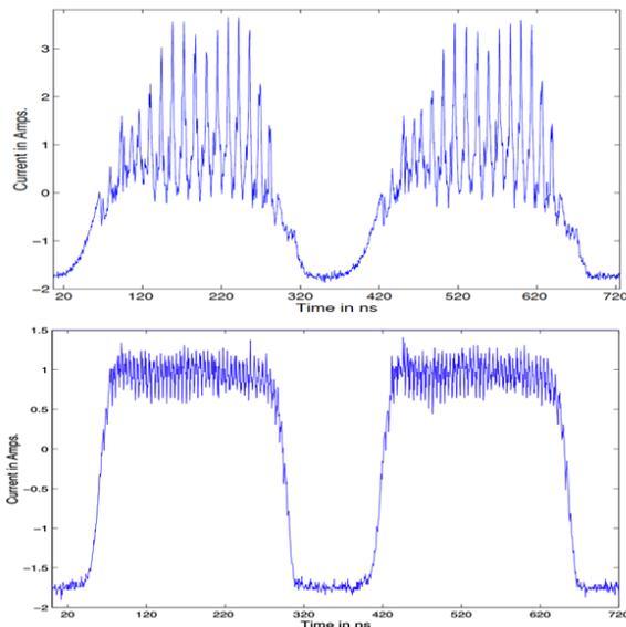
Figure 1: Two 300 ns beam pulses showing instability peaks (top). By heating the ferrite inductive inserts, the microwave instability is reduced (bottom).
