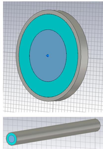
Figure 2: CST Microwave Studio Simulation of a single ferrite insert ring (top) and a 100 in long ferrite cavity mimicking the existing insert at the PSR (bottom).
