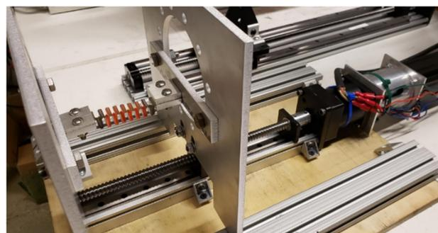
Figure 4: A custom fatigue tester constructed for this work.
