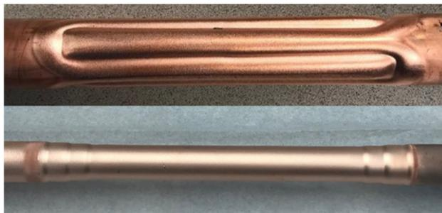
Figure 2: The erosion patterns produced by the stationary (top) and rotating (bottom) magnet packs.
