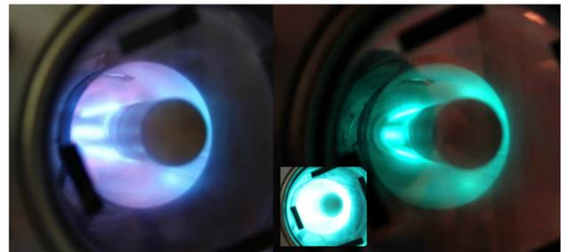
Figure 1: The first of two prototype magnetrons used for this work, shown here during an *in-situ* plasma etch/pre-clean step (left) and during a Cu dep (right) with a reduced exposure time due to the brightness. The inset photograph was taken with no reduction in exposure time relative to the photograph of the *in-situ* pre-clean step.
