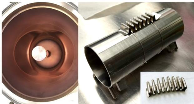
Figure 3: The sample holder (right) and the magnetron around which it mounted (left).
