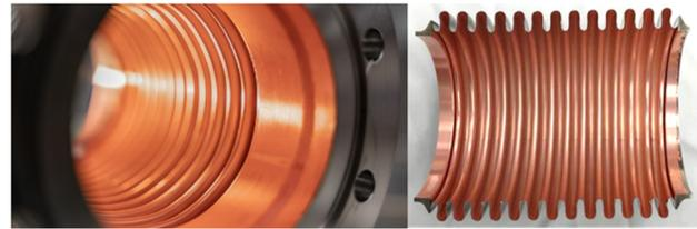
Figure 6: A photograph of the Cu-coated bellows and a cross section of the bellows prepared via wire-EDM.
