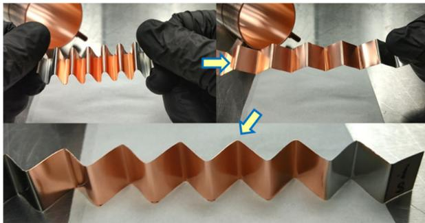
Figure 5: A sequence of images showing the plastic deformation of a substrate with a 5  $\mu\text{m}$  Cu film.
