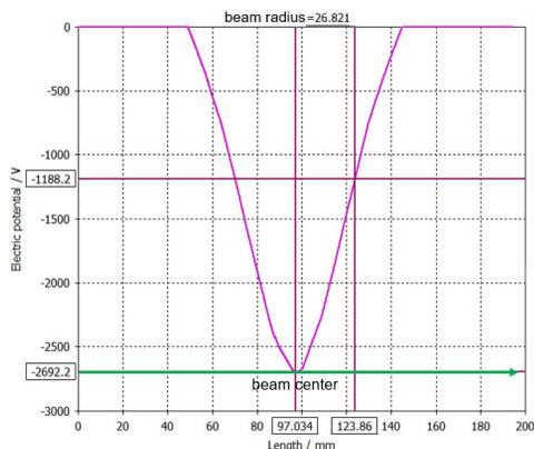
Figure 3: Space charge potential of the electron beam with 52 mm diameter at the location of the anode for 11 A current. Since the charge distribution is not uniform, the space charge potential is the maximum at the beam center and decreases non-linearly towards the edges. The potential is zero where the cylindrical anode is placed.
