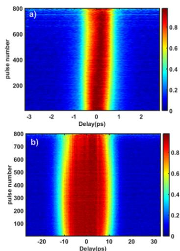
Figure 4: DUV pulse duration characterization by cross-correlation measurement for short pulse operation (a) and long pulse operation (b). Colour bar: Intensity of cross-correlation (normalized).
