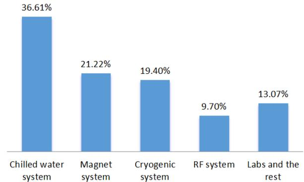
Figure 3: Energy usage percentage of different system in NSRRC 2020.
