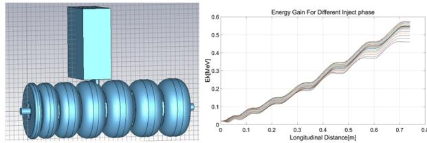
Figure 4: Vacuum model of the accelerating structure in CST (left) and kinetic energy evolution longitudinal(right).
