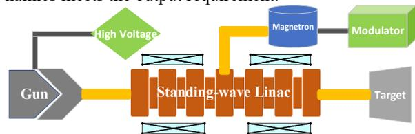
Figure 2: Layout of the designed linac system.
