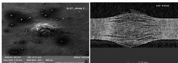
Figure 4: UKAEA SEM Results (left [16]) & CERN micro-CT scan (right) on the HRMT-43 Sigraflex<sup>®</sup> sample.
