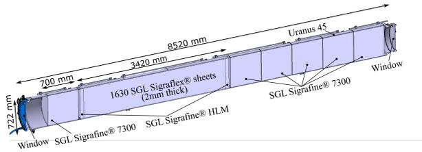
Figure 1: Schematic illustration of the TDE Dump.
