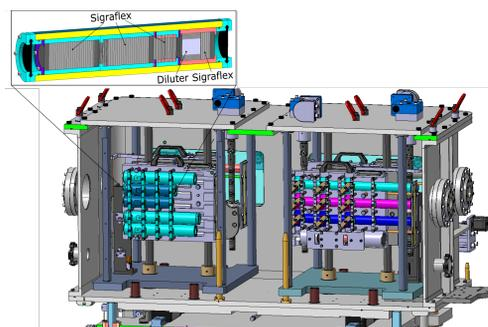
Figure 5: HRMT-56 (“HED”) tank and Sigraflex<sup>®</sup> target.
