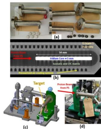
Figure 3: (a) Six manufactured Ti-6Al-4V external assemblies. (b) x-ray image of one of the targets equipped with  $\varnothing$ 3 mm Ir cores before its installation. (c) New target integrated in its module.
