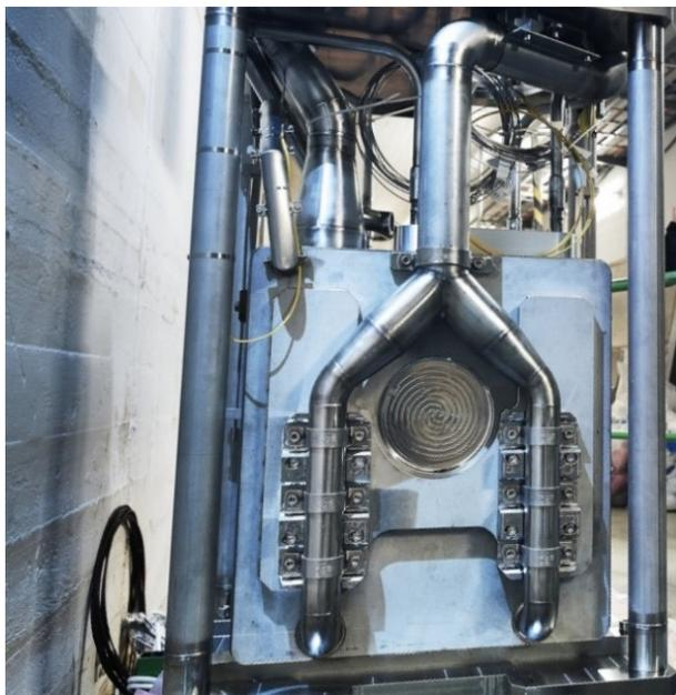
Figure 2: Third-generation n\_TOF target before installation in the beamline.
