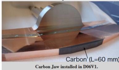
Figure 4: The jaw attached carbon.
