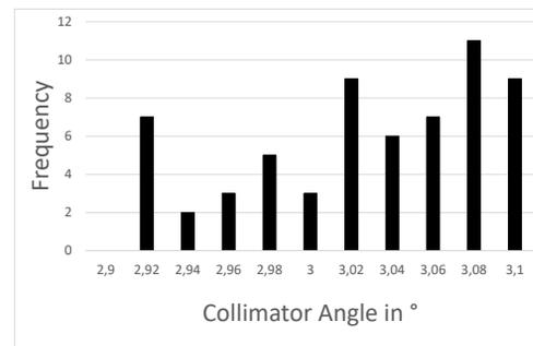
Figure 5: Frequency distribution of angles between beam axis and collimator block. The specification is  $3^\circ \pm 0.1^\circ$ .
