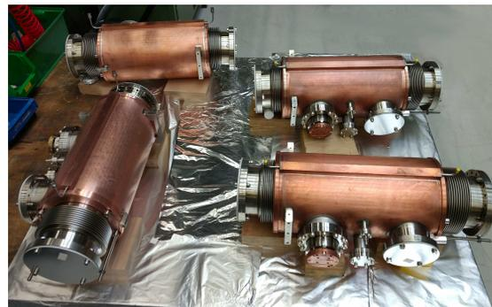
Figure 1: Series cryocatcher modules during site acceptance test at GSI.
