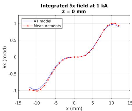
Figure 2:  $\theta_x$  deflection angle w/ respect to horizontal position: 1 kA supplied MIK (measurements: red, simulated data: blue).
