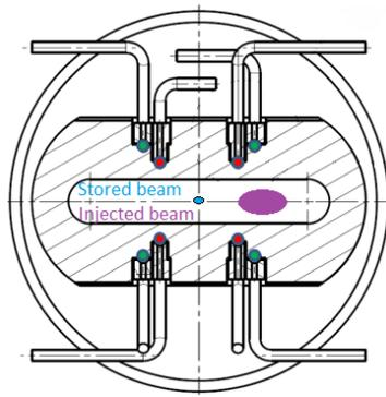
Figure 1: MIK cross section: red and green copper rods, striped sapphire vacuum chamber of the MIK (46.8 mm (H) x 7.8 mm (V)), purple injected and blue stored beams.
