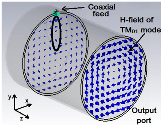
Figure 2: Process of  $TM_{01}$  mode generation through magnetic field coupling (waveguide shown transparent).
