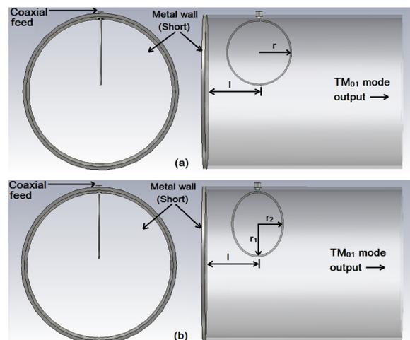
Figure 1: Front view and side view (waveguide transparent) of the proposed mode launcher with (a) circular and (b) elliptical loop feed.
