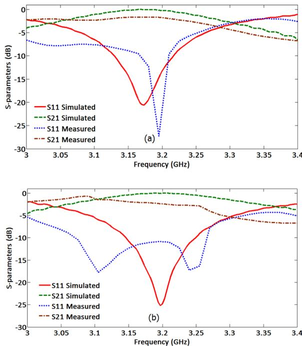
Figure 5: Measured S-parameters of the mode-launcher with (a) Circular and (b) Elliptical loop feed.
