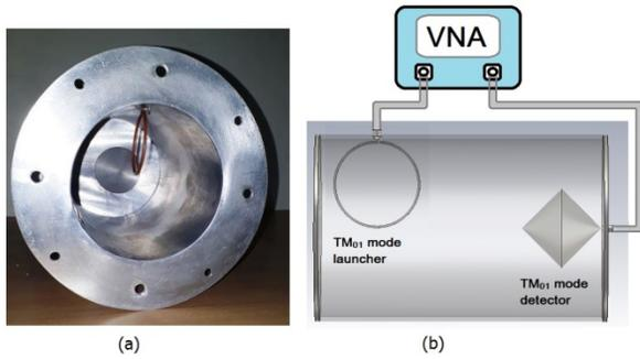
Figure 4: (a) Fabricated circular loop feed mode-launcher with biconical detector. (short metal plate removed for inside view) and (b) Illustration of measurement setup for circular loop feed mode launcher (waveguide shown transparent).
