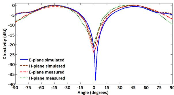
Figure 6: Measured radiation pattern (normalized) for the circular loop feed mode-launcher at 3.2 GHz frequency.
