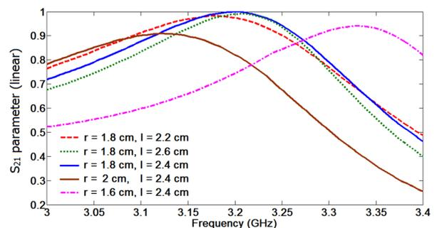
Figure 3: Effect of parametric variation on the  $S_{21}$  parameter of the mode-launcher with Circular loop feed.
