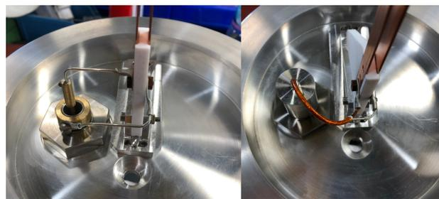
Figure 3: Two different options to connect the feedthrough to the probe loop. Left: using a homemade connection based on modified multicontacts. Right: Using an of the shelf connection solution.
