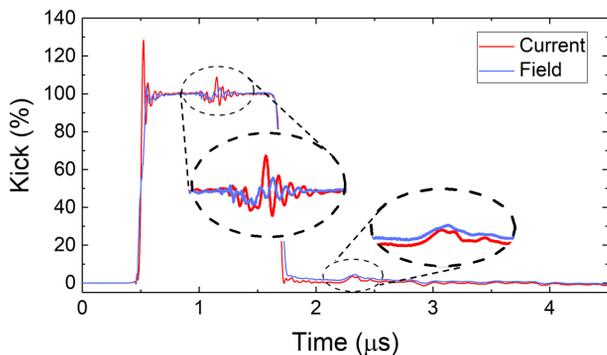
Figure 4: Normalized pulses comparison between current measured at the entrance of the magnet and the magnetic field measured with the probe plus the integrator.
