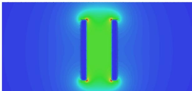
Figure 1: Magnetic field obtained when two parallel plates are simulated in Opera<sup>®</sup>2D.
