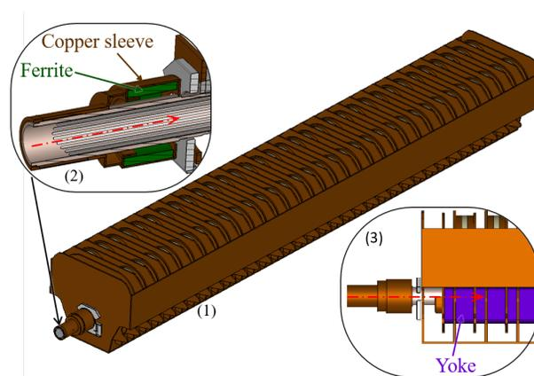
Figure 1: (1) The kicker magnet in its entirety, with the damper located on the left hand side. (2) Cross section of the damper (cooling pipes not shown). The red arrow indicates the direction of the beam. (3) External side view of the damper.
